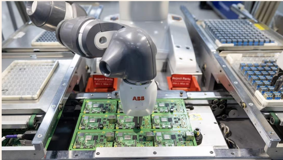
A robot places a component on a Raspberry Pi computer. The company began trading in 2012 and has sold more than 60mn single-board computers and computer modules © Bloomberg
